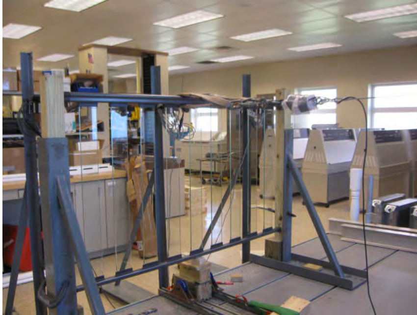
Photo No. 3 Horizontal Concentrated Load on the Top Rail
