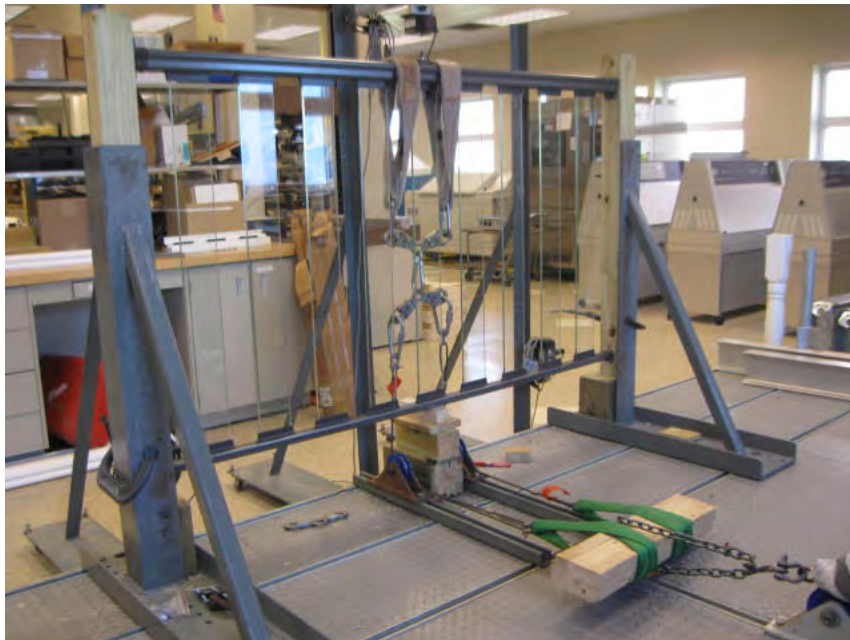
Photo No. 4 Vertical Concentrated Load on the Top Rail
