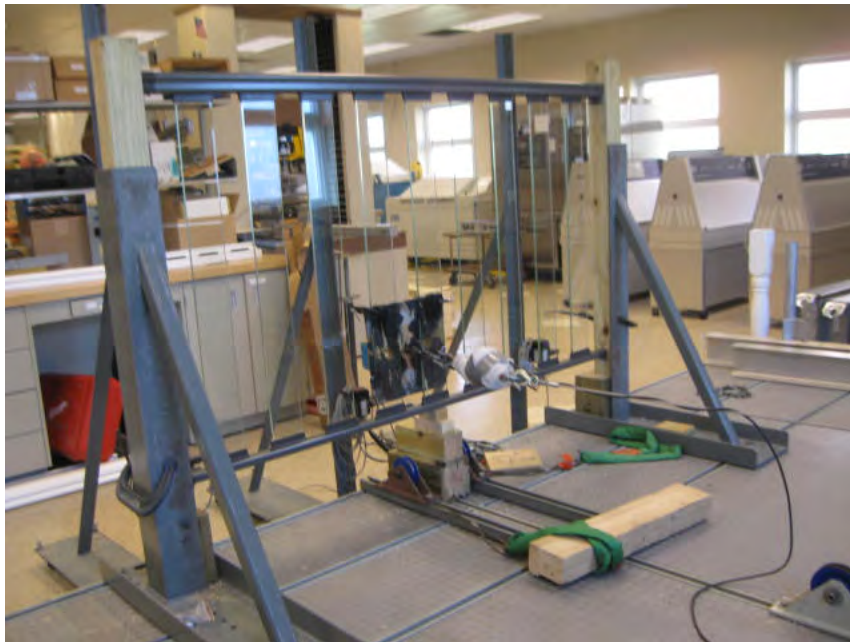
Photo No. 2 Load at Bottom of In-Fill
