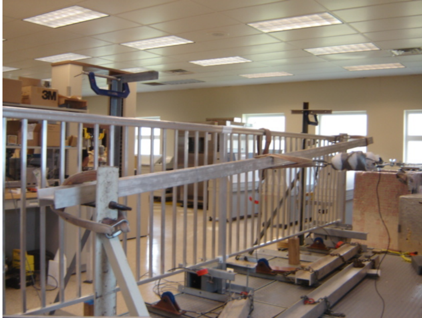
Photo No. 1 Test Method A - Specimen One Horizontal Concentrated Load on Top Rail Adjacent to 3-1/2 in Surface Mount Post
