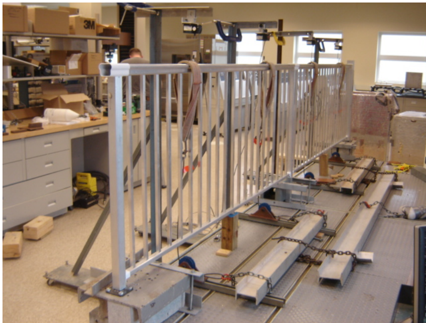
Photo No. 4 Test Method B - Typical for Specimens Two and Three Vertical Uniform Load Simulated by Quarter Point Loading of Both Top Rails
