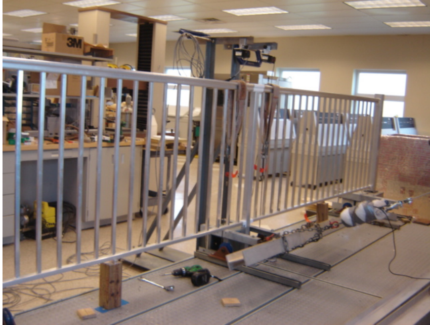
Photo No. 5 Test Method B - Typical for Specimens Two and Three Vertical Concentrated Load on Top Rails Adjacent to 1 7/8 in Side / Fascia Mount Post
