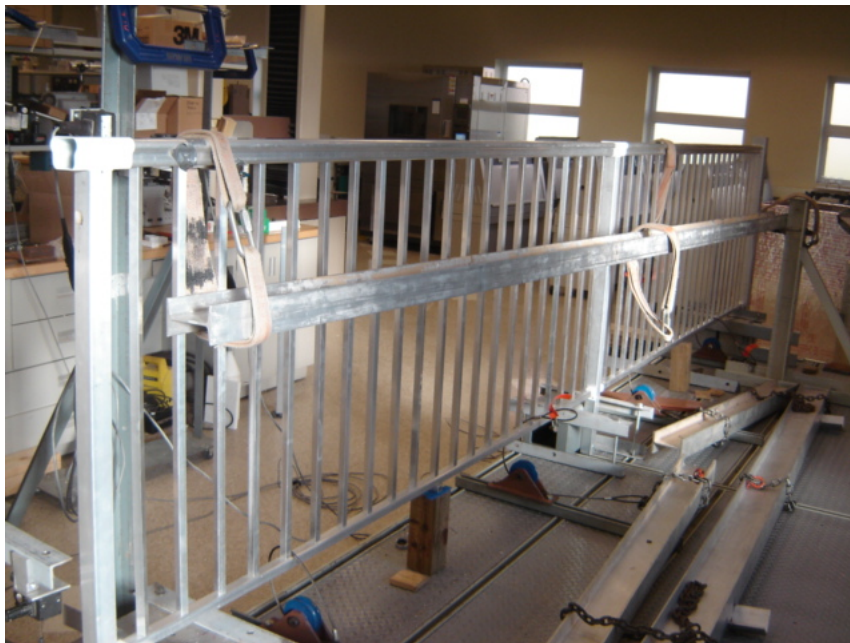
Photo No. 2 Test Method A - Specimen One Horizontal Concentrated Load on Top Rail Adjacent to 1-7/8 in Surface Mount Post
