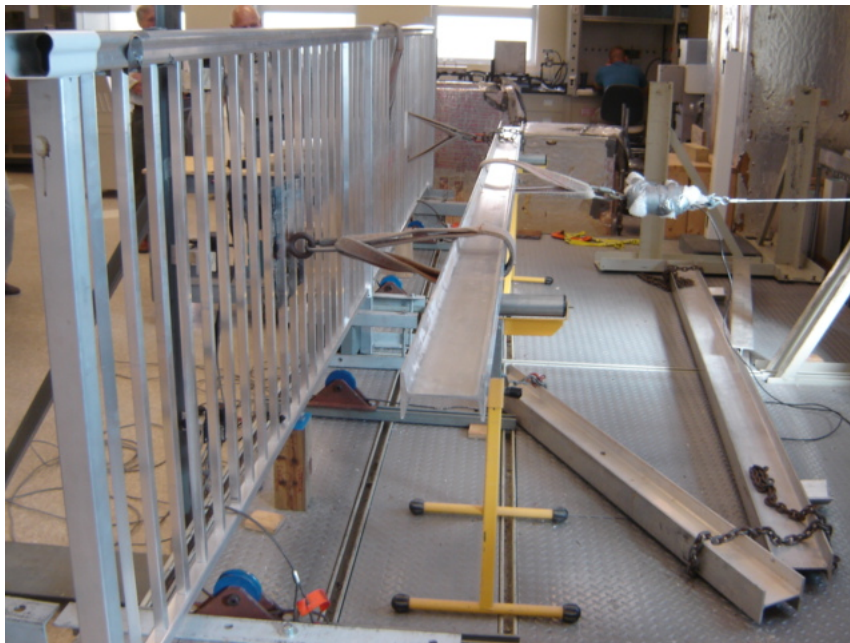
Photo No. 6 Test Method C - Typical for all Specimens Horizontal Concentrated Load on In-Fill at Mid-Height of Two Balusters
