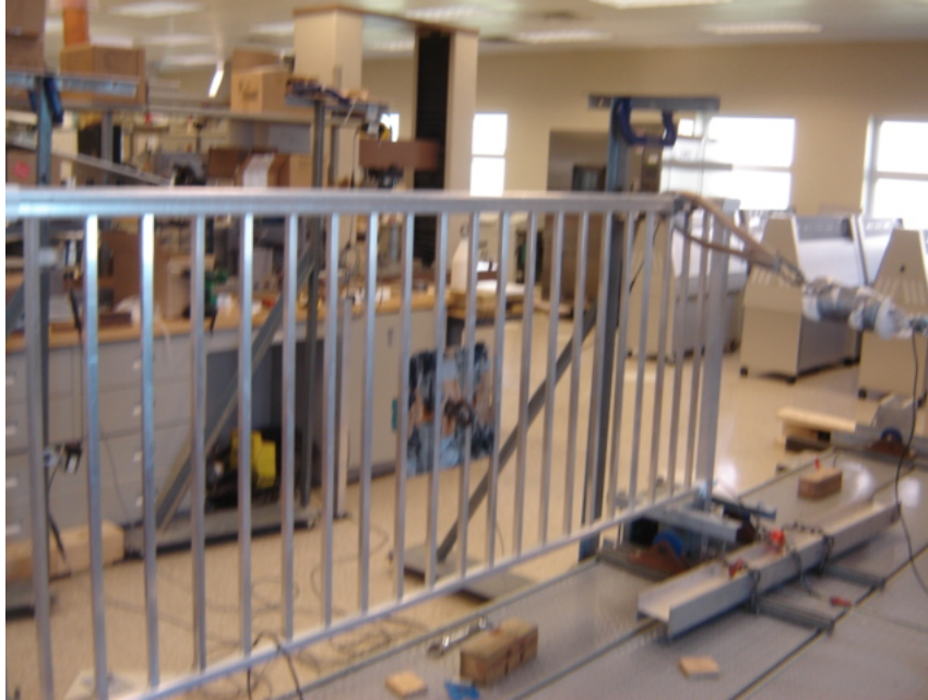
Photo No. 3 Test Method A - Specimen One Horizontal Concentrated Load on Top Rail Adjacent to 1-7/8 in Surface Mount Post with Right Guardrail Section Removed to Create an End Post Condition
