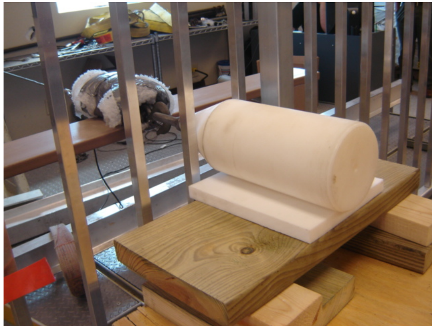
Photo No. 7 Test Method D - Typical for all Specimens Horizontal Load on Cone at Mid-Height of Two Balusters
