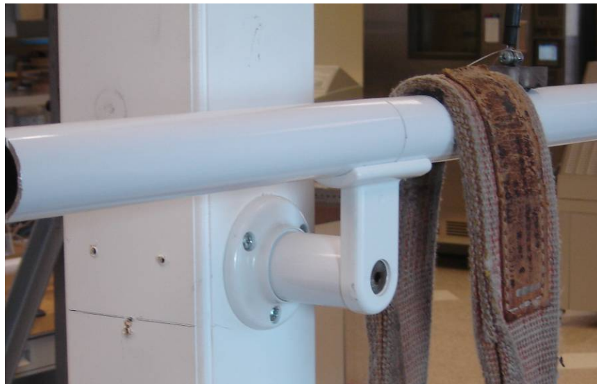
Photo No. 8 Mid-Rail Bracket, Spacer Tube, and Wall Mount Bracket Attached to Composite-Sleeved Wood Post
