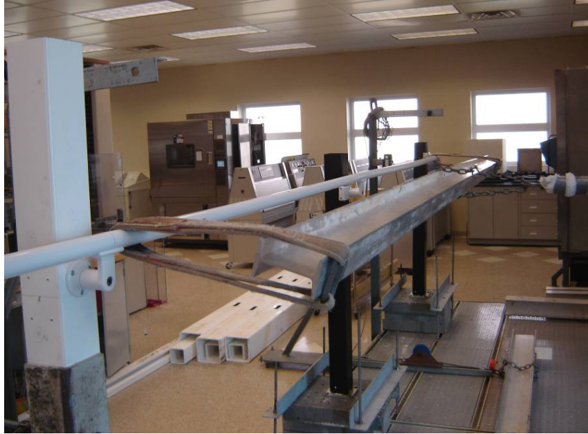
Photo No. 3 Test Method A - Horizontal Concentrated Load at Handrail Ends Adjacent to Brackets Specimen 1 of Configuration No. 2 Depicted
