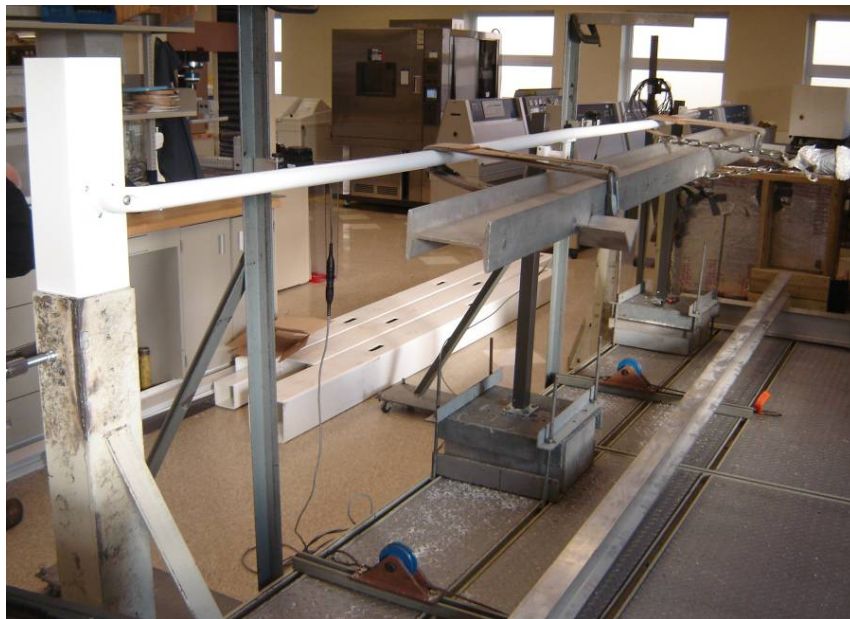
Photo No. 4 Test Method A - Horizontal Concentrated Load at Mid-Span of Each Handrail Section Typical for Specimens Two and Three - Configuration No. 1 Depicted
